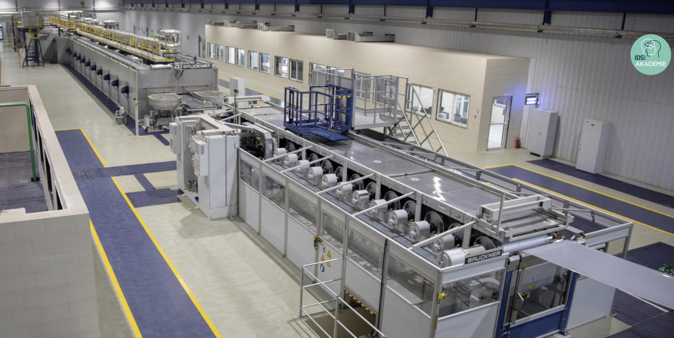
One of Brückners core products: film stretching lines.
